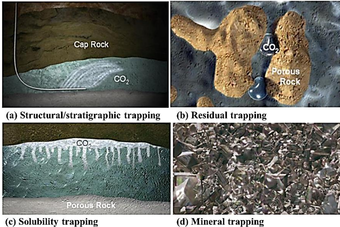
Figure 2-2: The four main CO 2 trapping mechanisms [81].
