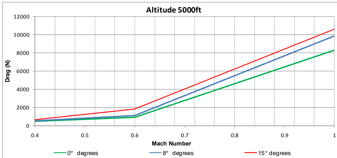
Figure 5-27: Drag vs. Mach number for different AOA
