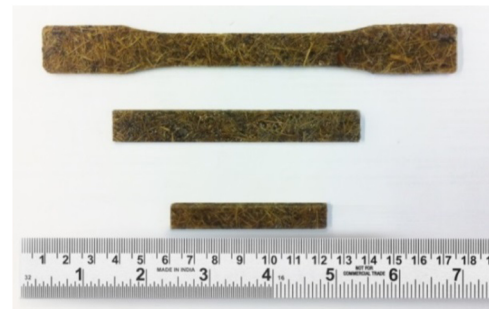
Fig. 3. 60% (w/w) AKF/PLA biocomposite specimens. Top: specimen used for tensile test. Middle: specimen used for three-point flexural bend test. Bottom: specimen used for impact test.
