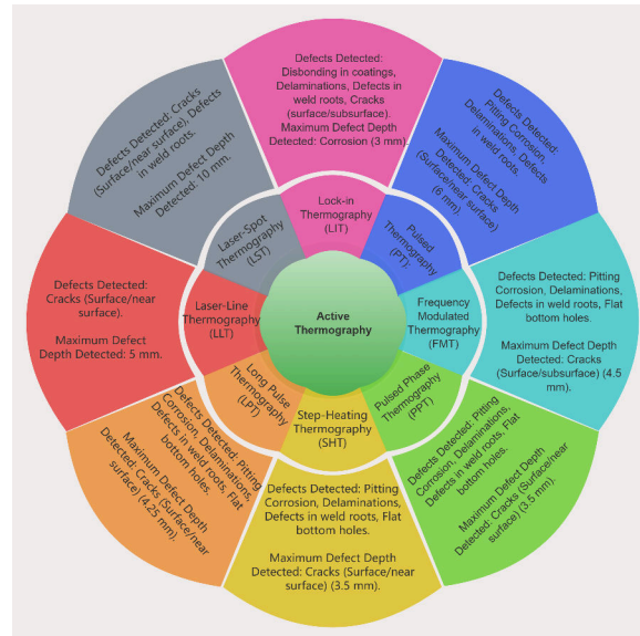
Figure 1. Overview of active IRT methods and empirical detectability guidelines (for sources, see Table 1).
