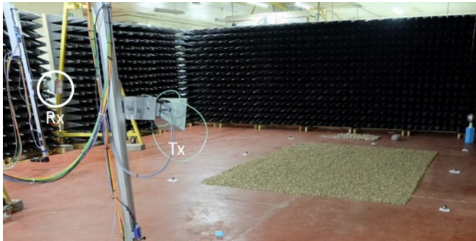
Figure 2. The GBSAR laboratory in a bistatic configuration, measuring a gravel scene. The locations of the transmitter (Tx) and receiver (Rx) are marked. Several metal spheres are positioned around the gravel to aid alignment checks.
