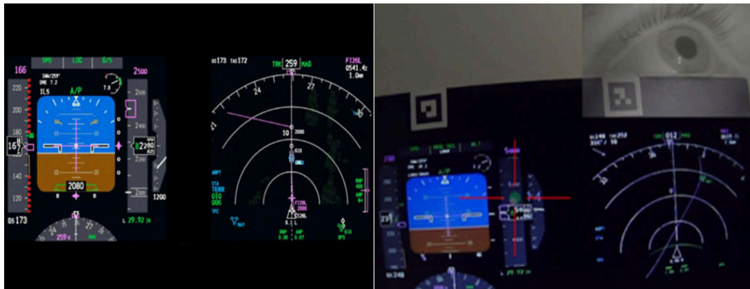
Figure 6. The images of PFD and ND captured by cockpit image recorder (left) versus pilot's fixations on the PFD with pupil dilation taken by eye tracker (right) providing specific information related to Human-Computer Interactions in flight operations
