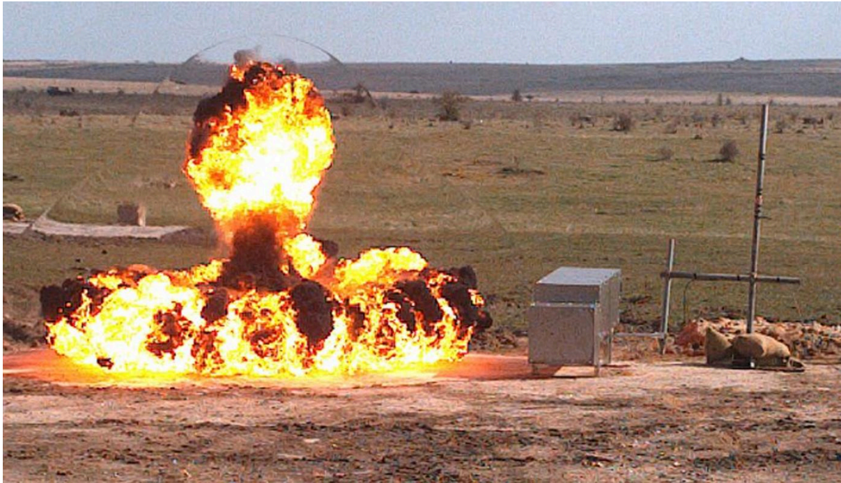
Figure 2 – Still from a high-speed video with the vehicle positioned 2.25m from the C4 charge
