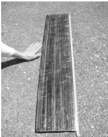
Figure 3: 1000mm x 200mm x 4 mm RUAM titanium wall structure
