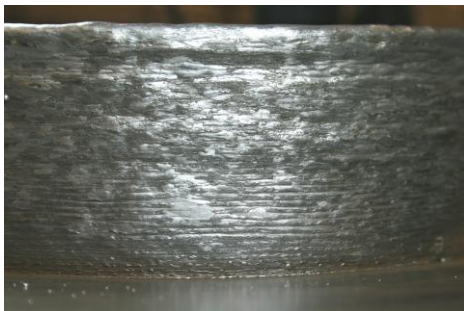
Figure 1: Layer structure of a wire based Additive Layer Manufacturing part
