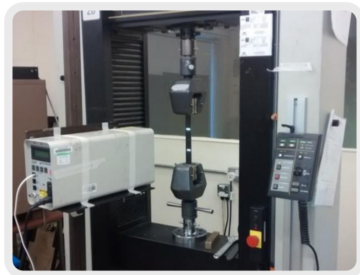
Figure 5-4. On-axis loading tensile test using Laser Electronic Instruments Research LE-05
