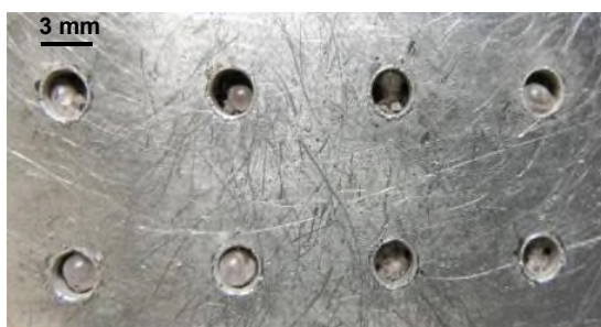
Figure 9. Bubbled RDX residues from ignited 1:1/4:1 large GNP samples. The scale bar represents 3 mm (hole diameter and depth).
