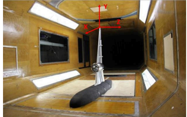
Fig 1: Wind tunnel model viewed from upstream
