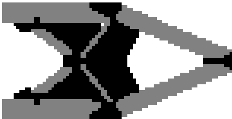
Figure 7 Aluminum occupies 25% of the design domain
