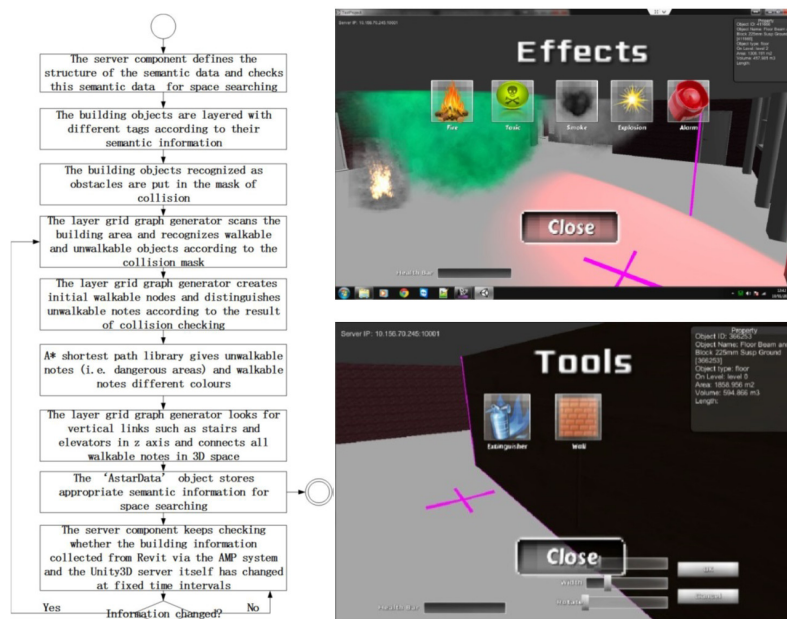
Figure 7. Workflow and tool library to create colored 3D scenarios in Unity server.
