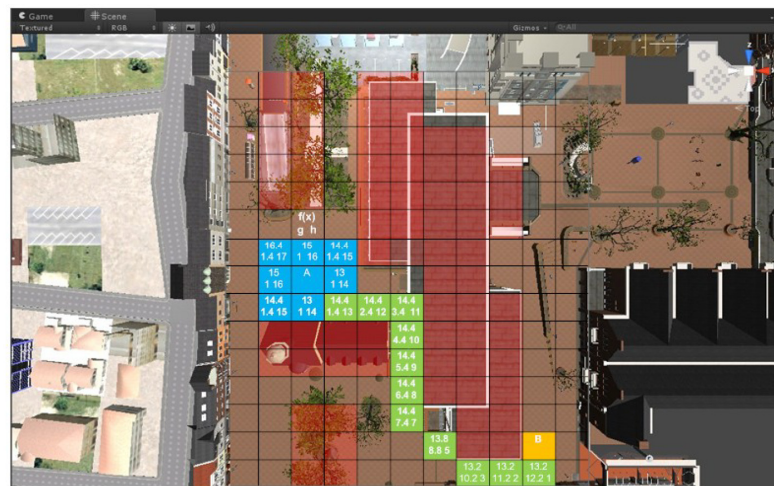
Figure 6. A* shortest path finding based on tile movement.
