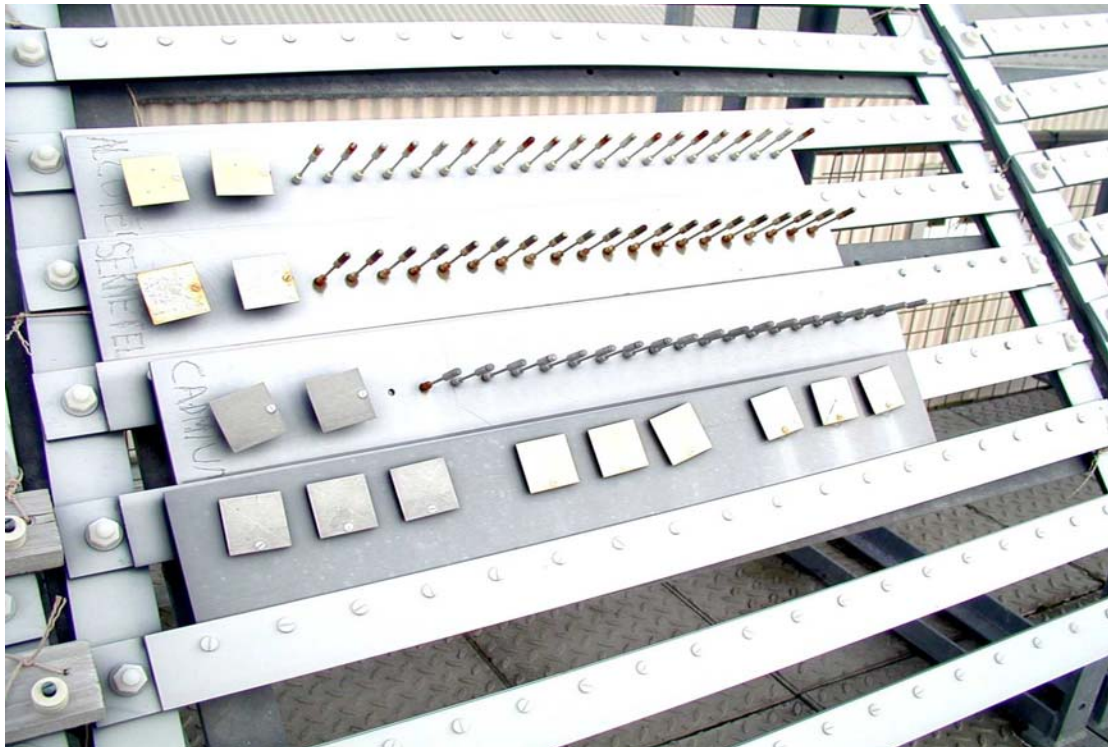
Figure 45. Arrangement of specimens and panels exposed to marine atmosphere.
