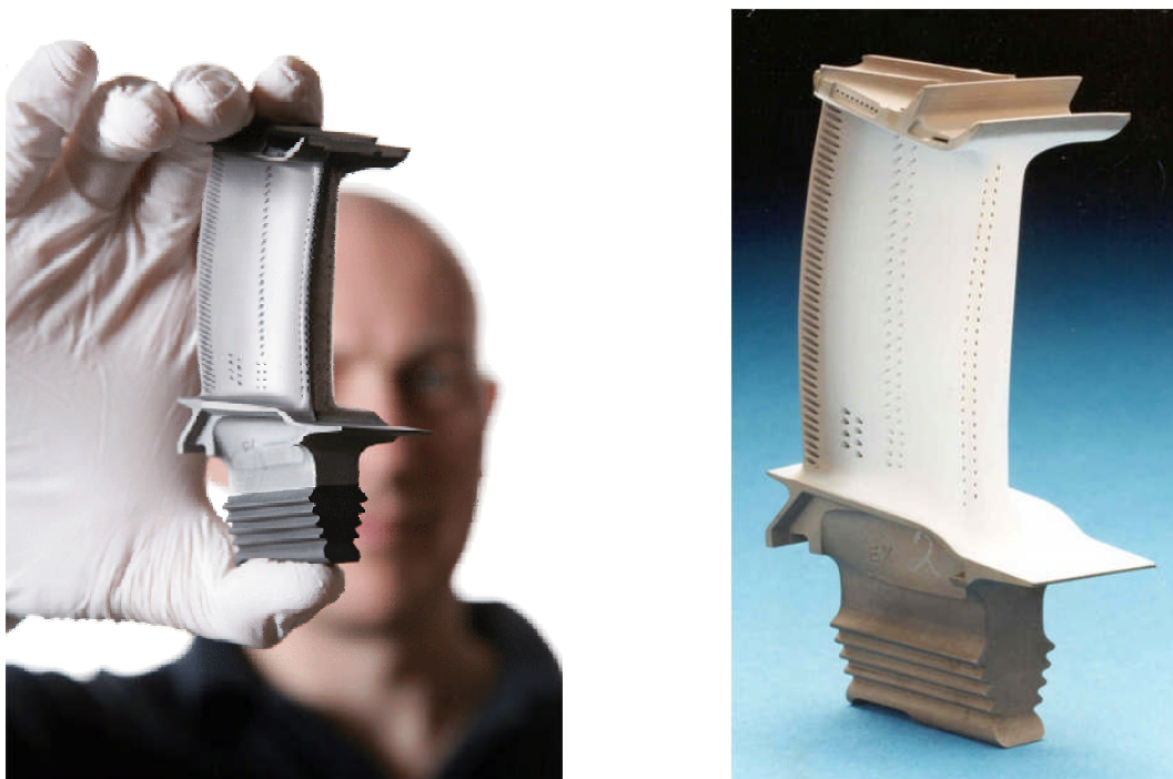
Figure 2. Rolls-Royce jet turbine blade with (a) ceramic coating (white) and (b) outlets for cooling air.
