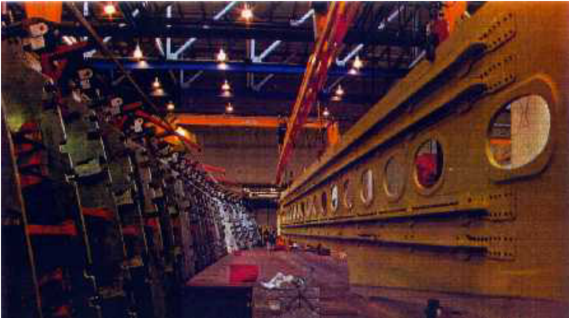
Figure 1.1 Wing stringers assembled on to the wing skin using the drill jig (Round, 1992)
