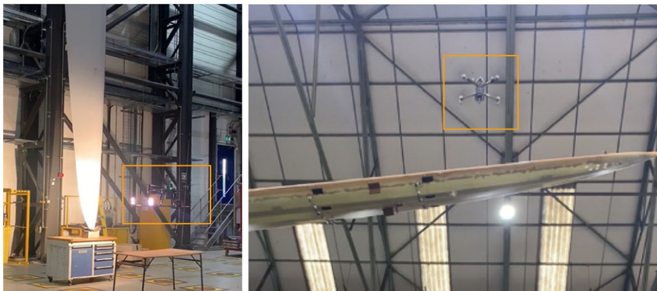
Figure 16. The UAV platform that performs active thermography inspection (three-day demonstration trial took place in ORE Catapult facilities in Blyth).
