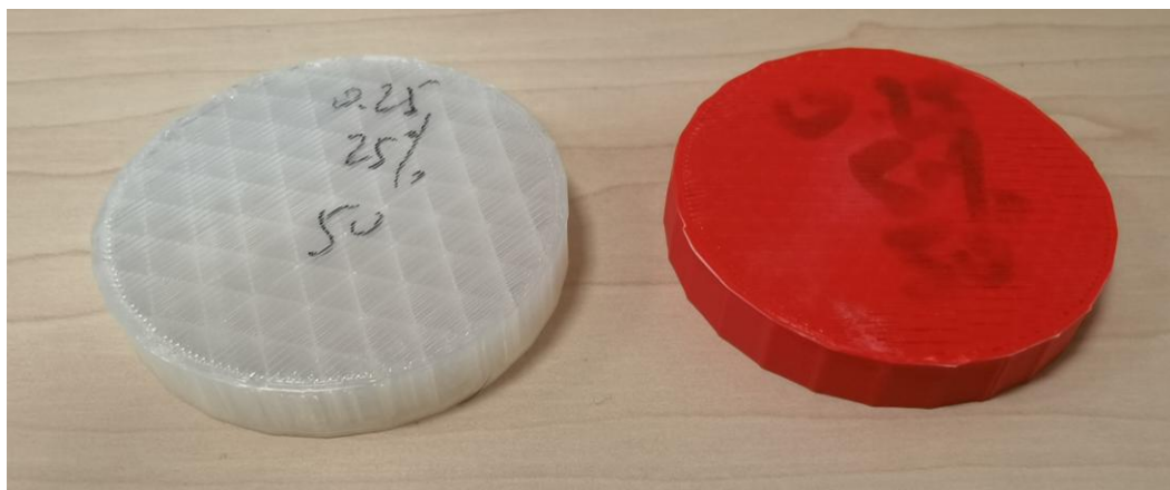
Figure 2. Two printed test samples. Left: PA12. Right: ABS.
