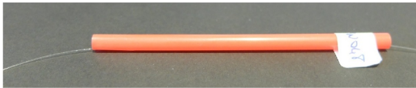
FIGURE 2 Dipole on a nylon monofilament protected in a length of drinking straw.
