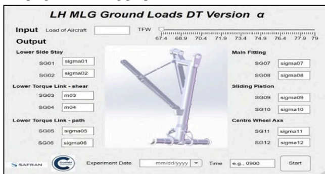
Fig. 5. MLG ground loads (force and torque) DT version \alpha interface
