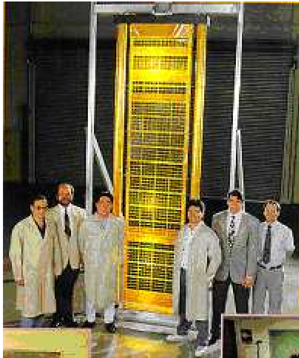
Figure B.7: Picture of L'Garde's 500 W solar arrays once inflated [L'Garde, 2003].
