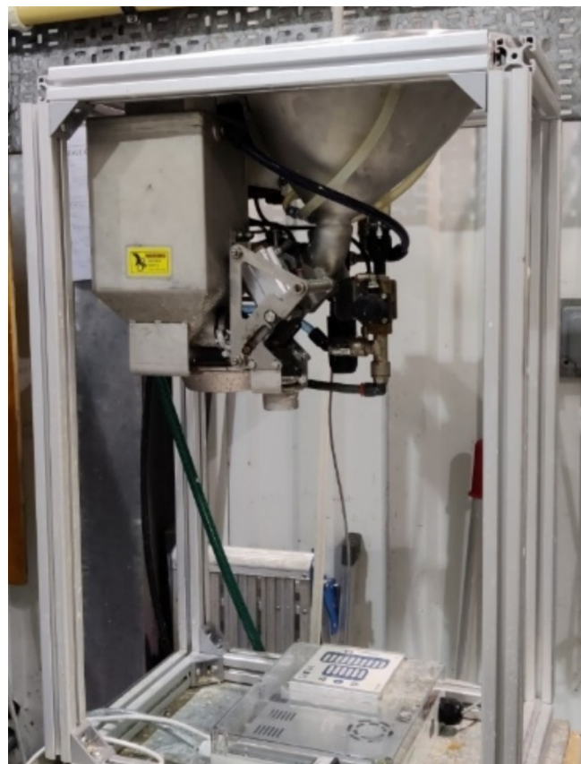
Fig. 1. Vacuum toilet set-up.
