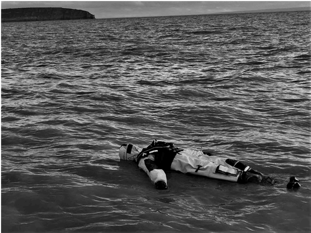
Figure 7 Training manikin (Dead Fred) being tested for appropriate flotation in the Bristol channel.
