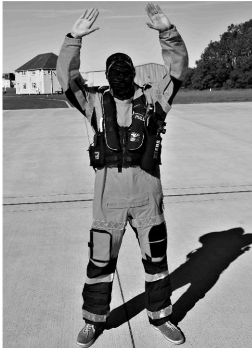
Figure 3 Configuration of retroreflective materials on immersion suit.
