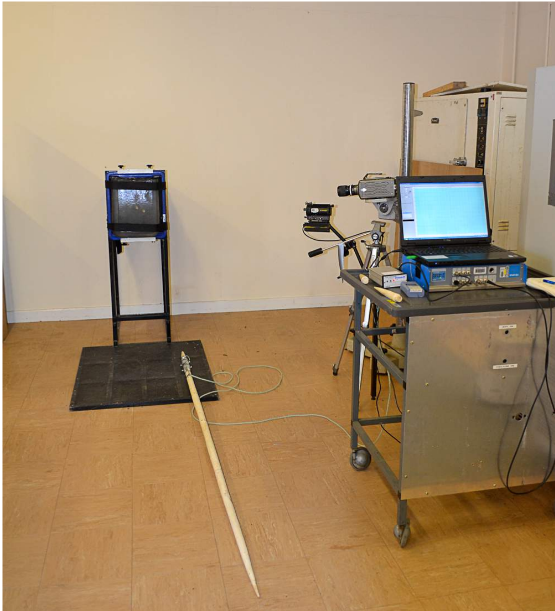
Figure 7. Experiment setup showing spear, PermaGel™ block, data acquisition and high speed video camera.
