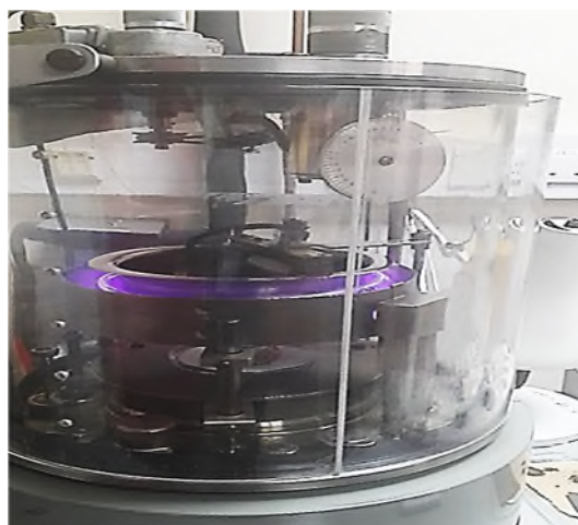
Figure 2-16: Glo plasma discharge to clean in-house TEM grids
