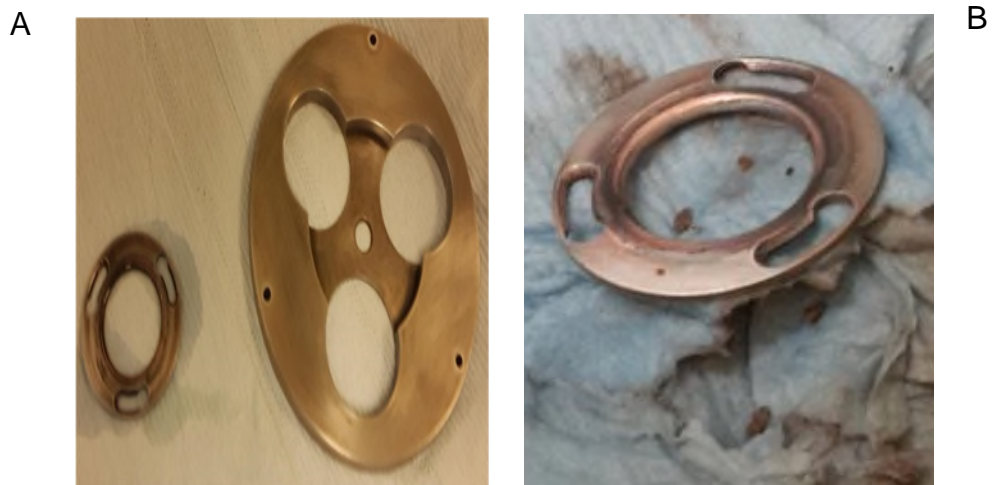
Figure 2-28: Target holders before (A) cleaned after sputtering (B).
