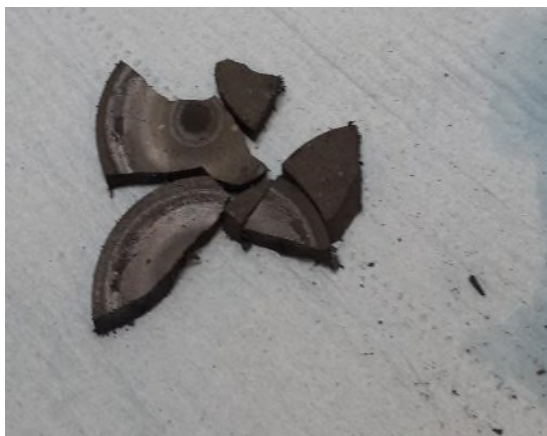
Figure 2-27: Broken iron oxide target.
