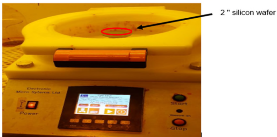
Figure 2-3: The spin coater used for coating the silicon wafer with PEG
