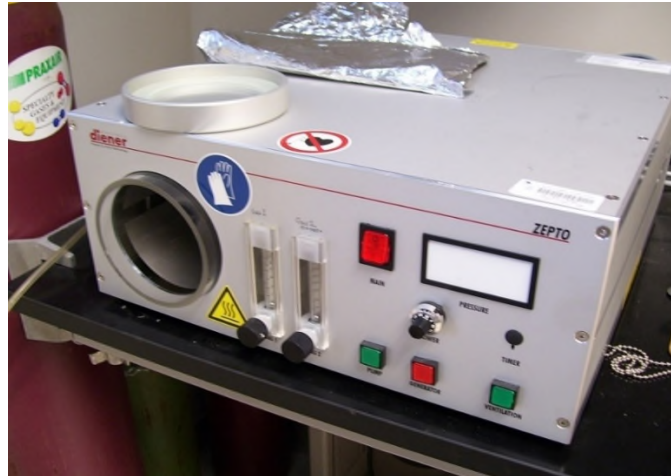
Figure 2-2: Plasma Cleaner prior to loading silicon wafer (Diener, 2022).
