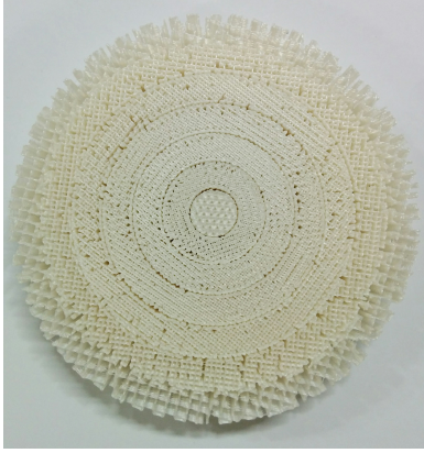
Fig. 4: Three-dimensional printed flat GRIN lens.
