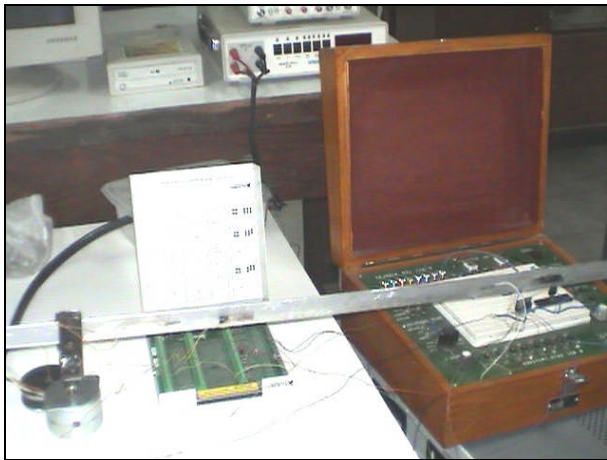
Figure 13. Experiment setup is showing flexible link with two IPMC actuators.
