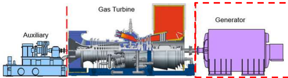
Figure 7: Hot End Drive (Aft of Gas turbine) (MHPS Gas Turbine Generator Set , 2015)
