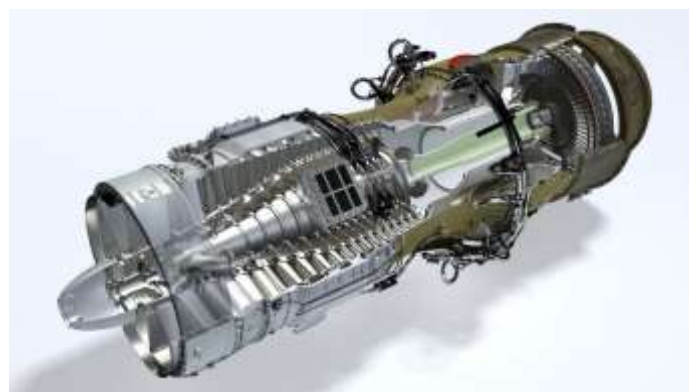
Figure 9: Roll Royce Avon Turbo jet engine (Advanced Animations UK, 2016)
