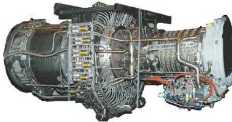
Figure 5: LM1800e aero-derivative engine (Gas and Steam Turbines, 2012)
