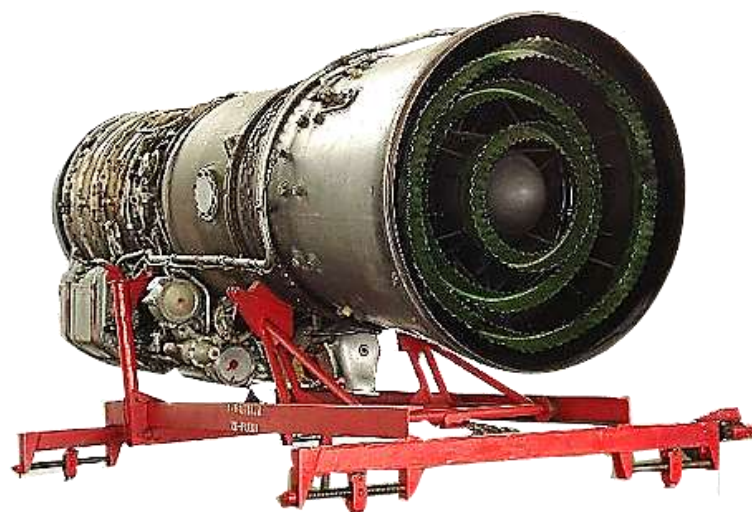
Figure 49: Tumansky- R25-300 turbojet engine on an engine mount (mm330046, 2007)
