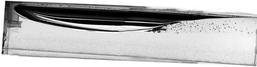
(a) Bubble shape from experiment, EXP1: VOL_{gas} = 0.001498m^3 , L_b = 0.2m , Fr = 0.4374
