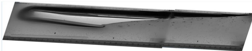
(g) Experimental Bubble shape for EXP5; 160cP oil, V_{so} = 0.32\text{m/s} , VOL_{gas} = 0.001498\text{m}^3
