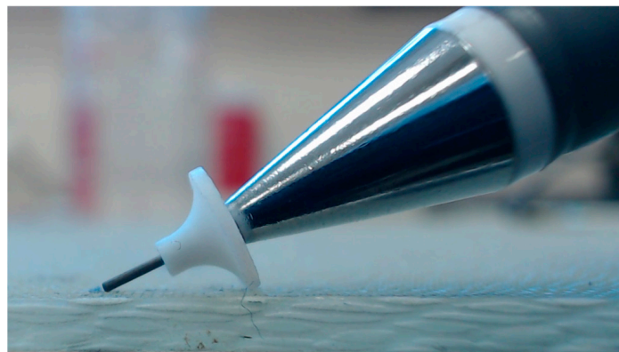
Figure 6. The pencil lead-breaking method.
