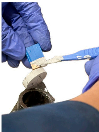
Figure 2. Applying cement coating to the sample to cover the wire connection.
