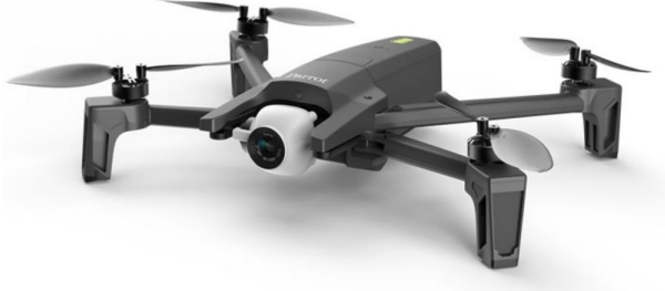
Fig. 2 Unmanned Air Vehicle, Parrot Anafi
