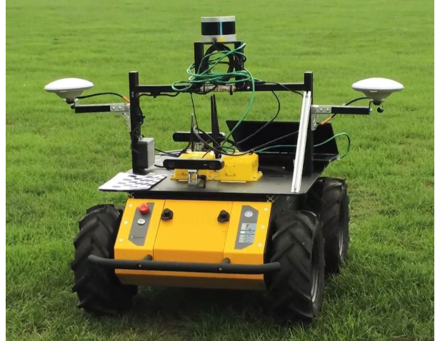
Fig. 3 Husky A200 Vehicle Platform snapshot with VLP 16 Lidar, Stereo Camera, Duro RTK GPS sensors payload (Centre for Autonomous & Cyber-Physical Systems, Ground autonomy Lab, Cranfield University)
