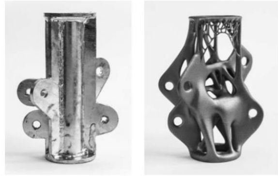
Figure 2. Node models: traditional way (left), 3D printing method (right) (Galjaard et al. , 2015a).
