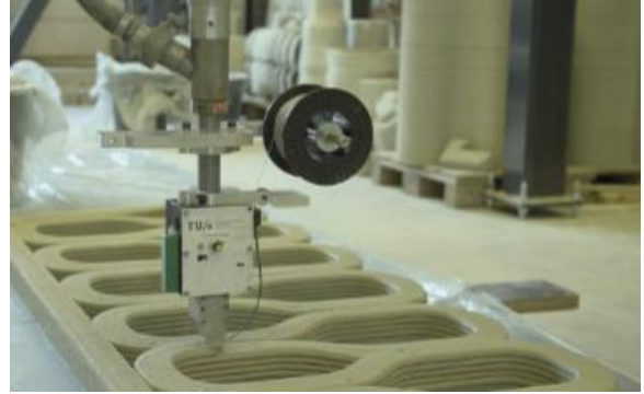
Figure 7. Material extrusion system (Paolini et al. , 2019).
