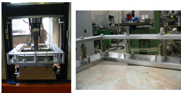
Figure 1: Forming apparatus for helicopter pilot mouldings, with (right) segmented blank holder.
