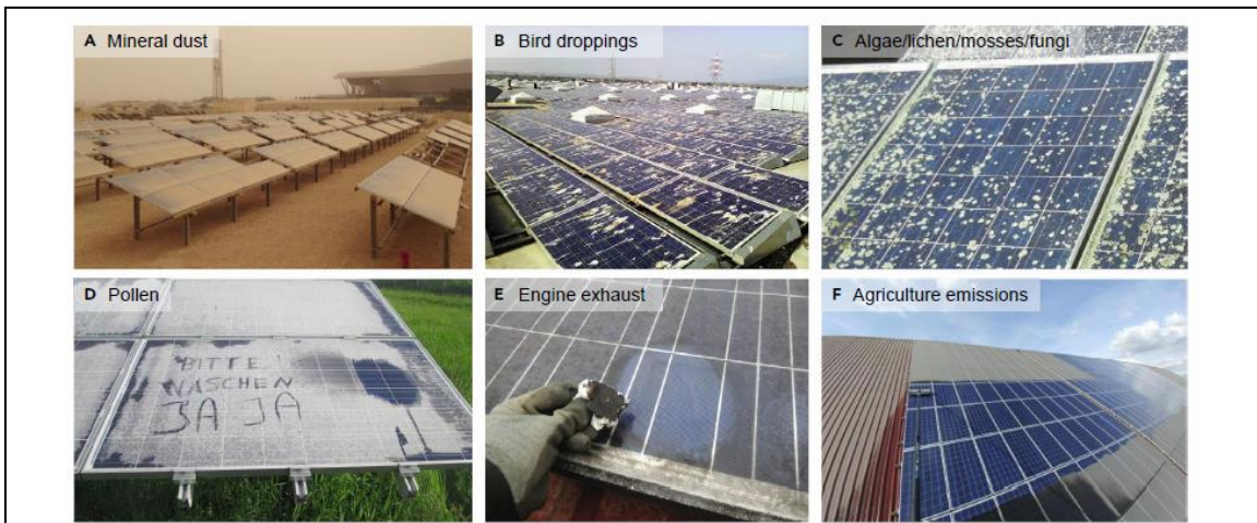
Fig. 7: Examples of intense soiling material of different types, (A) mineral deposit, (B) bird droppings, (C) biofilm of bacteria, algae, lichen, mosses, or fungi, (D) plant debris or pollen, (E) engine exhausts or industry emissions, and (F) agricultural emission e.g. feed dust. Source: [33]
