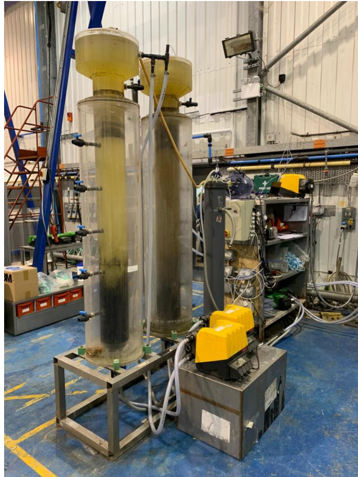
Figure B-1 Pilot-scale upflow anaerobic sludge blanket reactors.
