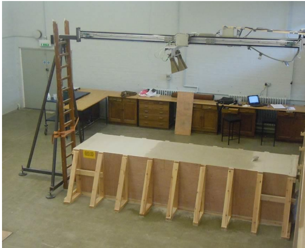
Figure 1: View of the laboratory, showing the linear scanner mounted centrally along the length of the sand trough.
