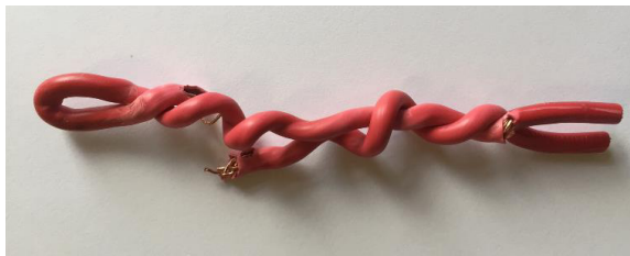
Fig. 12. An example of aged wire through twisting test process.
