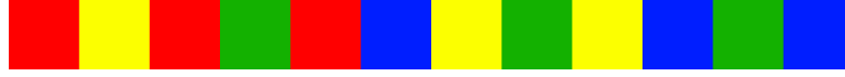
Figure 11: An example of De Bruijn sequence of order 2 over an alphabet of 4 symbols mapped to 4 colours with no repetitions. A sequence of 2 colors uniquely identifies a position.
