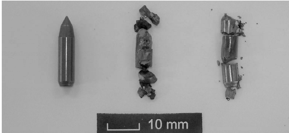
Figure 7: Recovered fragments of core after completely penetrating an 85 mm LPS SiC tile (middle) and a 33 mm LPS SiC tile (right). An intact projectile core is added for comparison (left).
