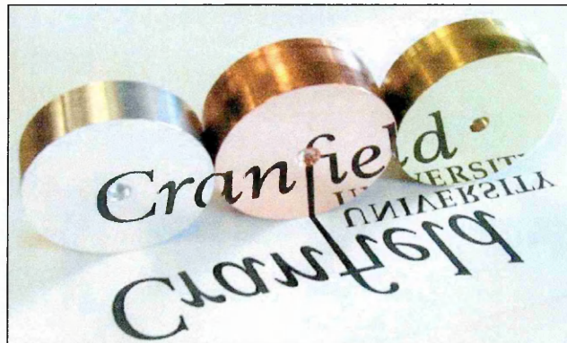
Figure 3-5: Diamond turned samples
