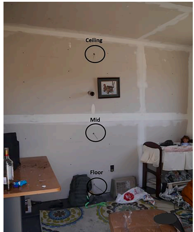
Fig. 2. Internal thermocouple placement.
