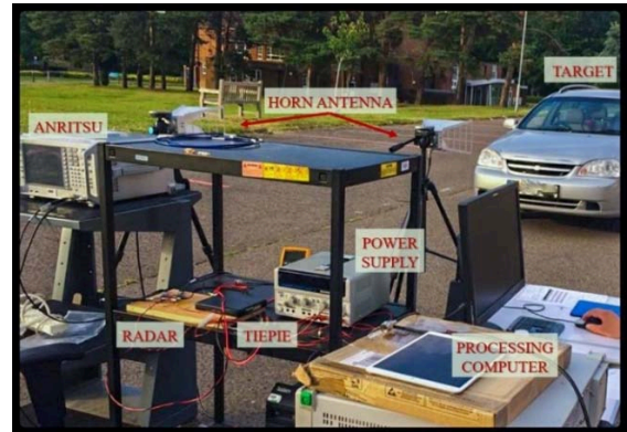
Fig 4: Radar Arrangement for Field Test
