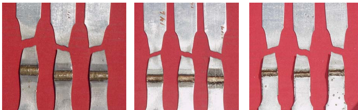
(a) (b) (c) Figure 6. Tensile Specimens for a) GMAW-Pulse using ER CuAl-A2 filler wire; b) GMAW-Pulse using ER CuSi-A filler wire; c) Variable polarity GMA braze weld using ER CuSi-A.
