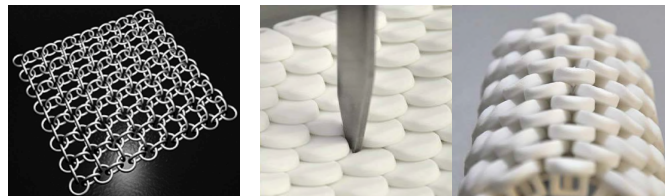
Fig. 36. Additively manufactured chain mail (left, [44]) and laser sintered articulated stab-resistant armor (right, [162]).
