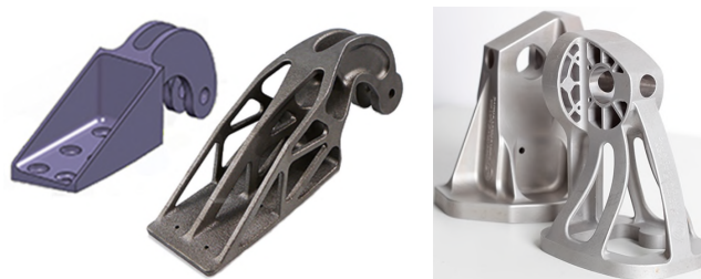
Fig. 16. Brackets before and after topology optimization: Airbus A320 nacelle hinge brackets as-designed for cast steel and optimized for titanium (left) and Airbus A380 brackets as designed and optimized for stainless steel (right) [105]. The optimized brackets were produced by direct metal laser sintering (DMLS).
