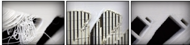
Fig. 43. Closeup of build support strategies: failed build with no support (left), successful build with support (center), and successful build of self-supporting structure (right). Adapted from [185].
