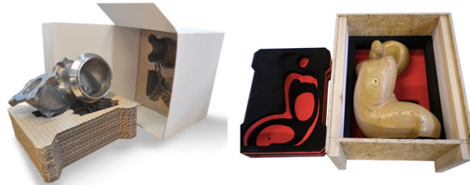
Fig. 22. Examples of products with custom-fit packaging: metal industrial component with cardboard packaging (left) and wooden sculpture “Océane” by Dominique Pollès with alternating polystyrene and foam layers (right) [34].
