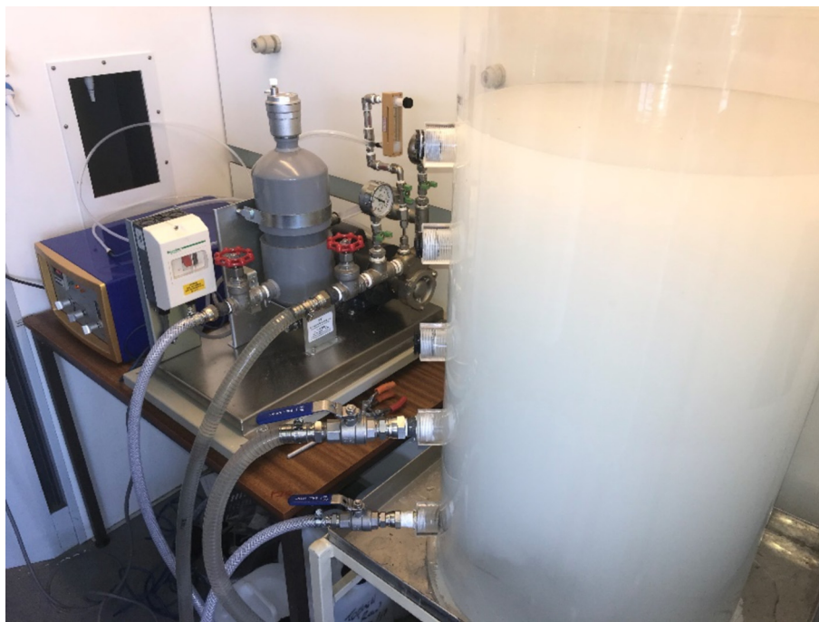
Fig. 1. Microbubble generation experimental apparatus.
