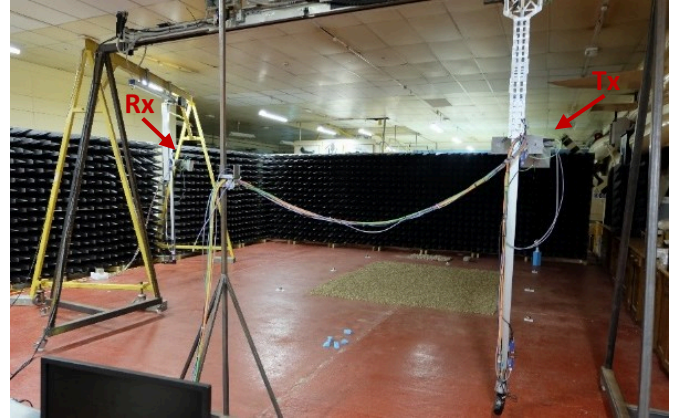
Fig. 1. The GBSAR laboratory in a bistatic configuration.
