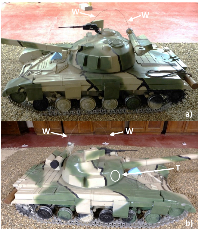
Fig. 9. Close-up side-views of the quarter scale T72 tank model. The highlighted parts are the arched antenna wire “W”, and the bistatic specular reflection point on the turret “T”.
