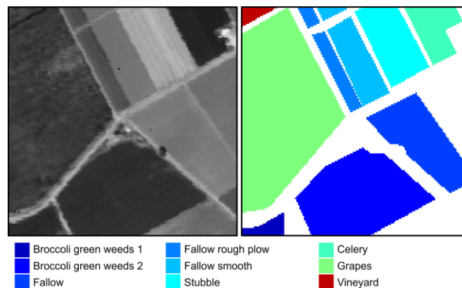
Fig. 6. One band image at the wavelength of 667 nm (left) and the ground truth map (right) for the Salinas C data set.
