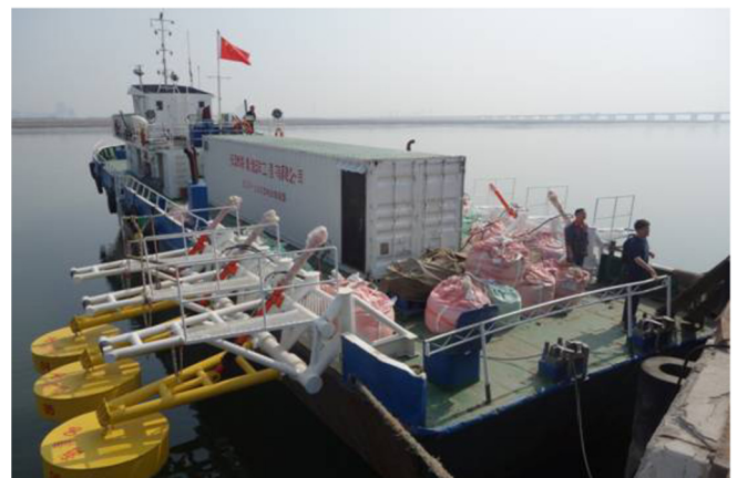
Fig. 2. Photograph of the NOTC 10 kW multiple-point-absorber WEC.
