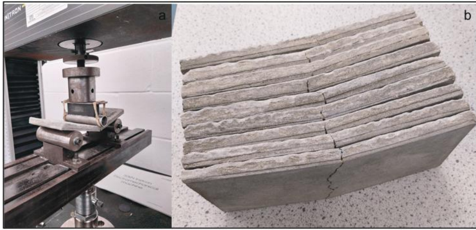
Figure 5. (a) Bending test machine applying load on specimen (b) a cross section of fractured specimen after bend test.
