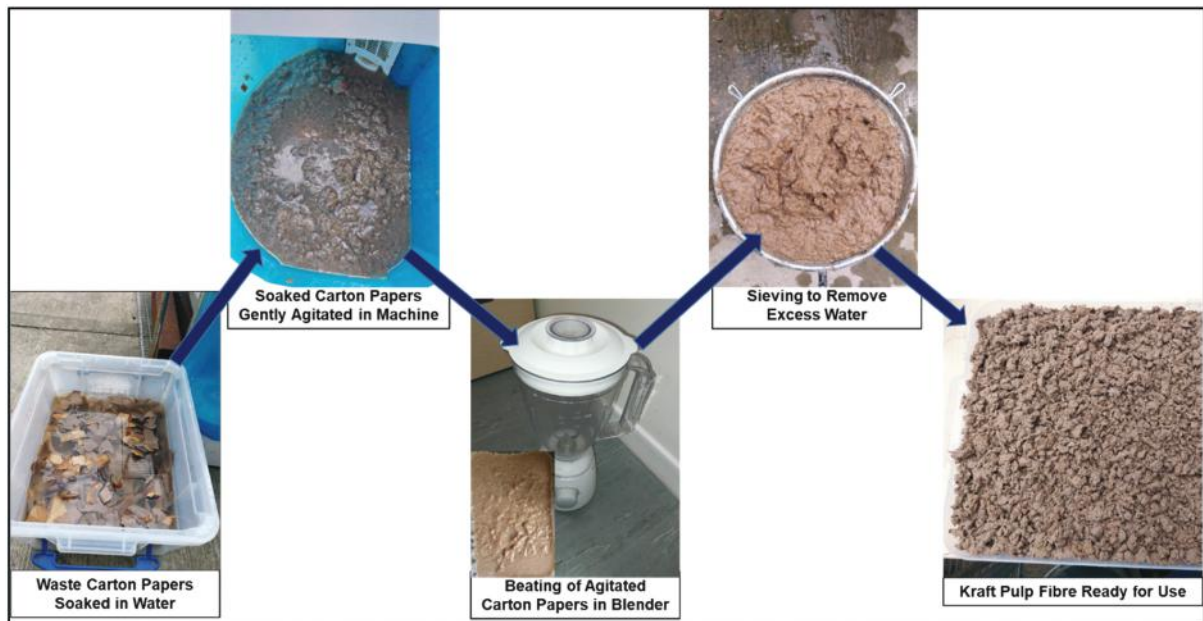
Figure 3. Series of images showing the process of obtaining the kraft pulp fibre.
